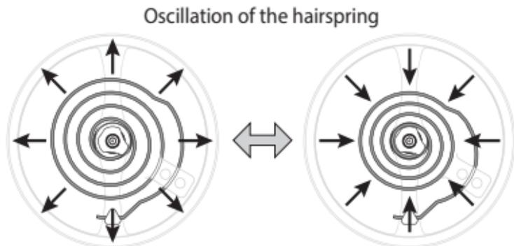
Oscillation of the hairspring may fluctuate and total movement of a mechanical watch is consequently affected much if a thing with strong magnetism exists its nearby.
